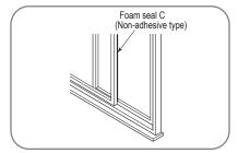
3. Cut the non-adhesive foam seal C strip to match the width(or height) of the window. Insert the seal between the glass and the window frame to prevent air and insects from getting into the room.
