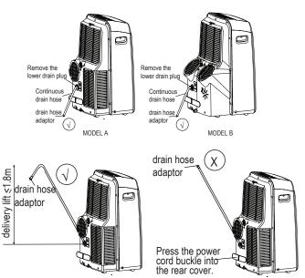
· (For model A1)During heating pump mode, remove the lower drain plug from the back of the unit, install the drain connector(5/8" universal female mender) with 3/4" hose(locally purchased). Carefully move the unit to a drain location, and let the water drain away. Note: Make sure the drain hose is lower than the
